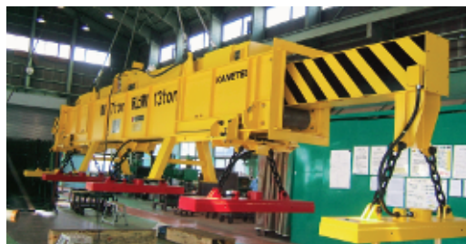
(Lifting steel plates)
