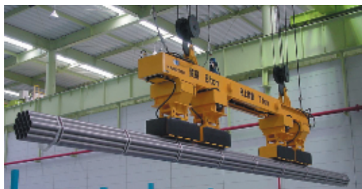
(Lifting bundled pipes)
