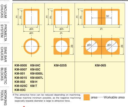
The attractive force can be reduced depending on machining. Please machine minimum possible, as the negative machining especially towards diameter is large to attractive force.
