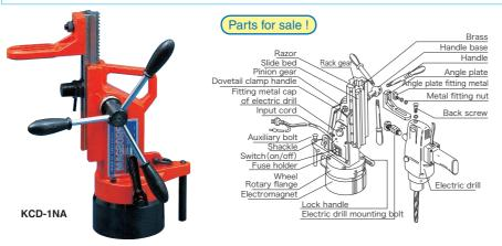
Circular magnet is turnable up to 320°. You can even drill thin steel sheet by placing backing material beneath the sheet
