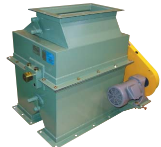
An example of fabrication of drum magnetic separator
