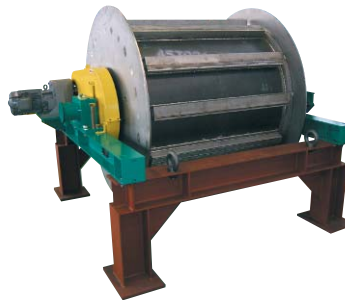
An example of fabrication of large electromagnetic drum
