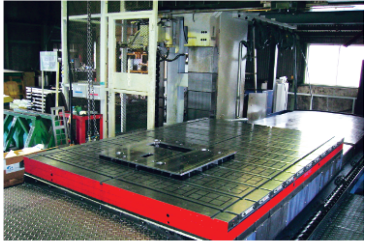
Permanent electromagnetic chuck for cutting (An example of large size)
