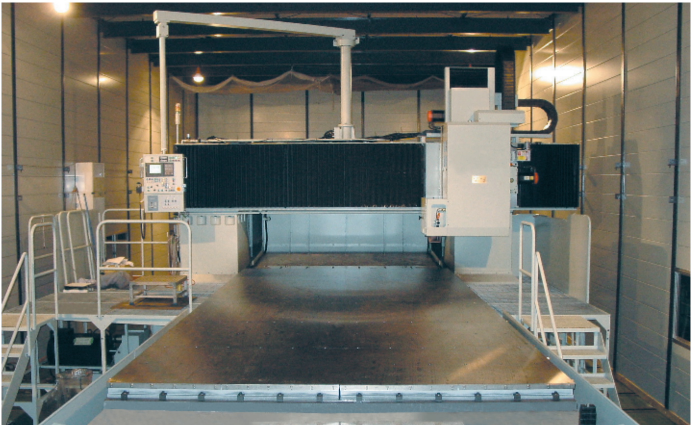
Permanent electromagnetic chuck for grinding (An example of large size)
