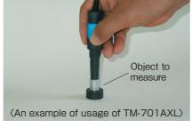
●A probe dedicated to TM-701. Please keep this probe as a spare; it can be replaced without troublesome calibration. In addition to the standard PRB (transverse type), an axial type (AXL) capable of measurement in the vertical direction and having higher durability is optionally available.
