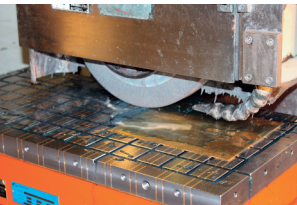
An example of grinding of brass by utilizing the permanent electromagnetic feature
